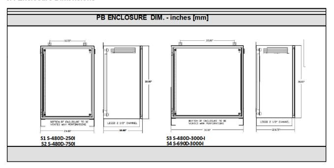
Phaseback/Silencer Voltage Transformer Size Y or Delta Industrial or Marine PB/HS 480/690 250/750/3000/6000 Y or D I or M
