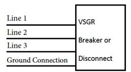
Connect Phaseback DVS to the motor to be protected with (3) #10 phase conductors and a #10 ground wire as shown below.
