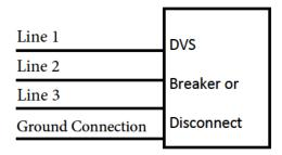
Connect Phaseback HS to the power source to be protected with (3) #10 phase conductors and a #10 ground wire as shown below.
